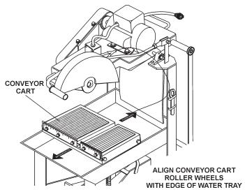
Figure 8. Conveyor Cart Placement
